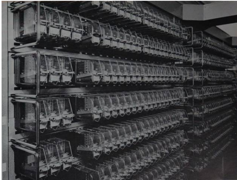
Figure 189 - SGE geographical interlocking, Paddock Wood. © Alstom.
