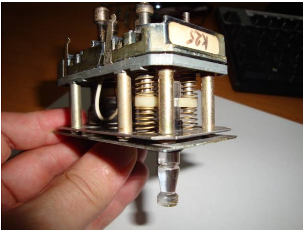
Figure 149 - Westinghouse M3 NX(PP)[+] tile top unit showing push-button assembly. © Brian Hornsey
